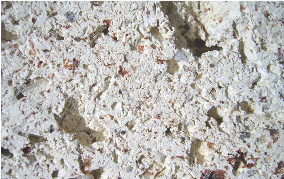
Enlargement : cross section of a rock with pores, cavities, fissures.
